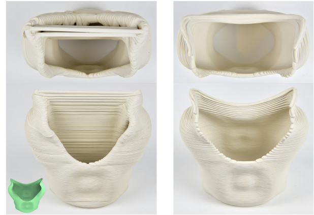
Fig. 2. Left: A strictly continuous path generated by Hergel et al. [2019]. We tailor this method to surface models by slightly thickening the original surface into a model with a valid volume. However, the redundant non-model structure still needs to be used to connect separate components of the model (see the top view). Right: Our toolpath is fully continuous due to the use of curved layers, without requiring an extra path.
