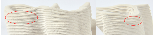
Fig. 19. The thickness was non-uniform in the outer boundary of the curved layers because the material deformed in different ways when extruded in the downhill or uphill directions.
